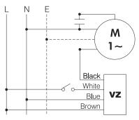
Single phase motors above 1.25 Amps and all three phase motors
